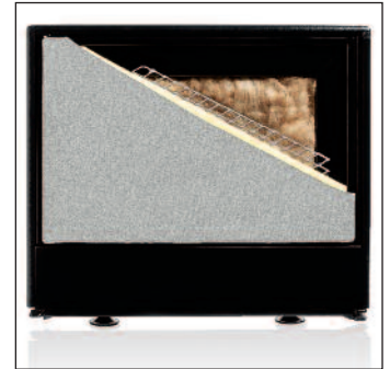
The steel frame and expanded metal skeleton of a System XXI panel core enclose acoustic barriers of fiberglass for a combination of panel strength and acoustical privacy.
